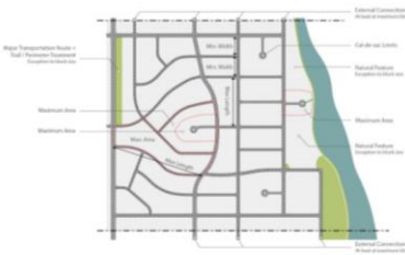
Figure 3-1: Connectivity & Block Sizes. Street layouts shall be based on maximum block size length between centerlines of perimeter streets and area and adjust to property at a frequency sufficient to create connected networks unless exceptions justify not connecting.
