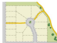
Figure 3-3: Walkways and Bicycle Routes. Where streets do not connect or larger blocks are patterned, connections for pedestrians or bikes may be required through blocks or at the end of disconnected streets (17-3-1.5).
