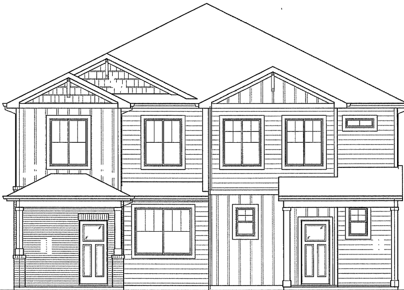
Front Elevation - Building Type (DT07 + DT08) 'D' SCALE: 1/4"=1'-0" AT 22'X34' LAYOUT 1/8"=1'-0" AT 11'X17' LAYOUT
