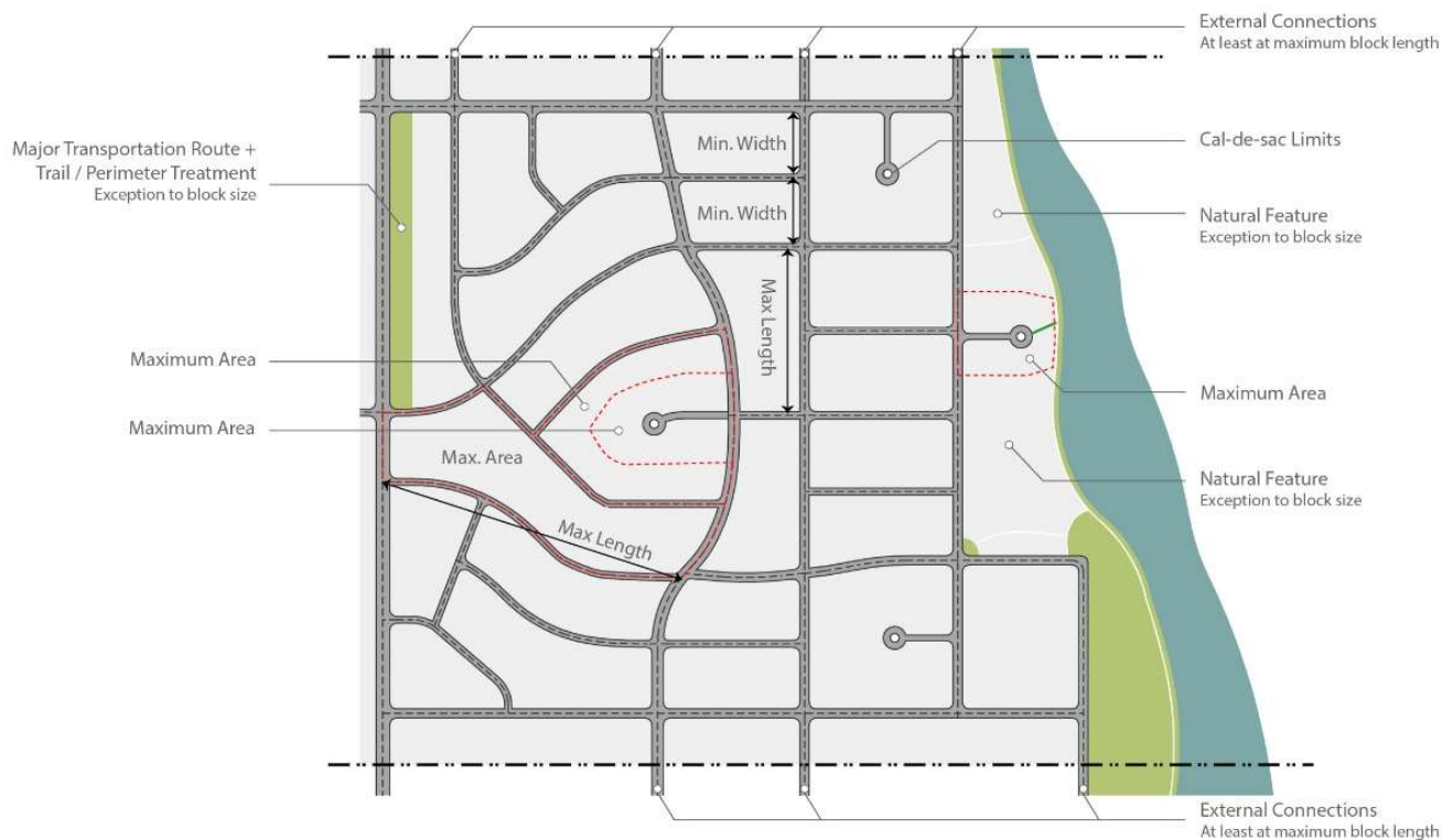
Figure 3-1 Connectivity & Block Sizes. Street networks shall be based on maximum block sizes (length between centerlines of perimeter streets and area) and stub to adjacent property at a frequency sufficient to create connected networks unless exceptions justify not connecting.
