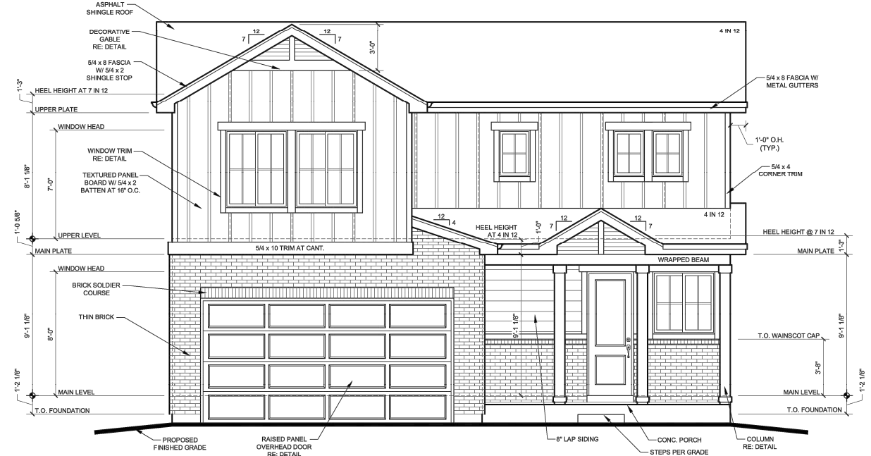
1 FRONT ELEVATION - 'A' SCALE: 1/4" = 1'-0" FARMHOUSE 33% MASONRY 15% GLAZING
