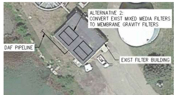
Figure 2: Alt #2 – Convert Existing Filters to MGFs
