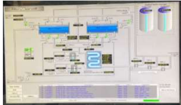
Photo: JWTP Filter / Clearwell SCADA Screen
