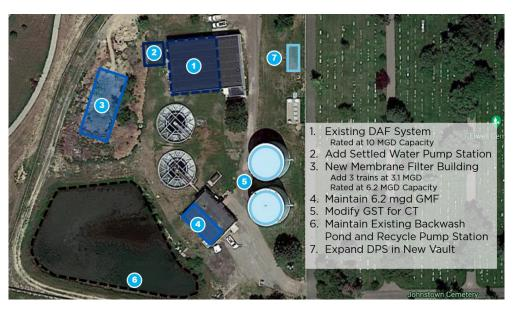
Figure 2-7. Option 2 - Membrane Filtration Addition
