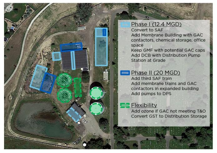
Figure 2-12. Potential Phasing Plan
