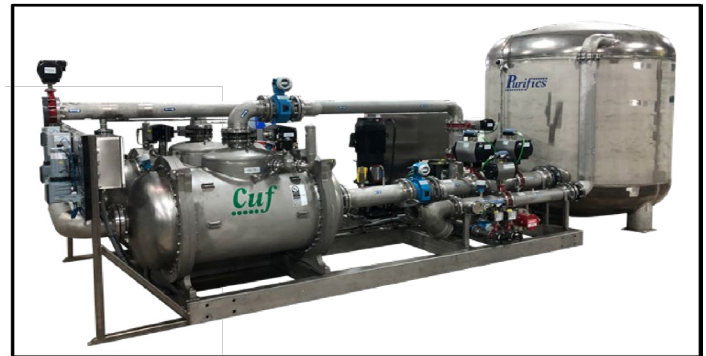
Ceramic membranes have been demonstrated to operate at flux rates of 250 gfd compared with 30 to 40 gd for polymeric membranes.
