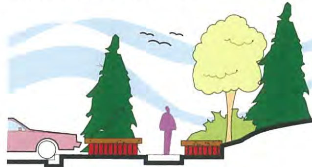
USE SCREEN WALLS, RAISED PLANTERS OR OTHER DEVICES TO PROTECT LANDSCAPING FROM PEDESTRIANS AND AUTOMOBILES.
