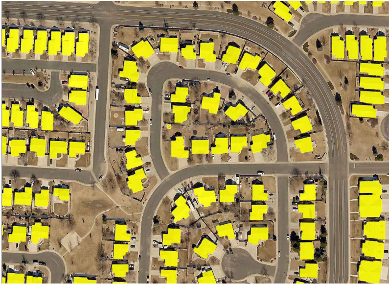
Roofline data for more than 8,500 buildings was generated by deep learning algorithms.
