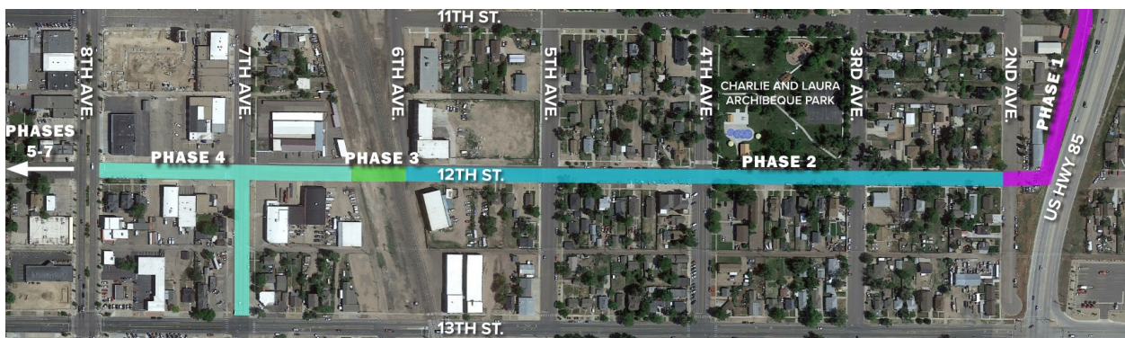
A phasing plan was developed for the 12 th Street Outfall during the master plan. Phase 1 is currently under construction with final design of Phase 2-4 underway
