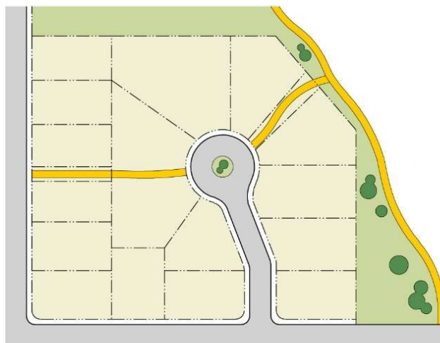
3-4 Walkways and Bicycle Routes. Where streets will not connect or where larger blocks are platted, connections for pedestrians or bikes may be required through blocks or at the ends of disconnected streets. (17-3-1.B.3).
