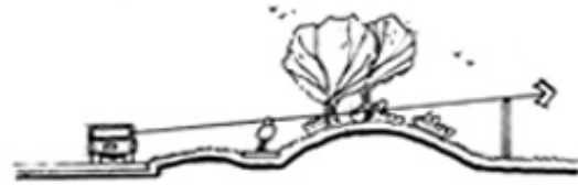
Figure 10-2 - Buffering Example for Chain Link Fence along a Public Right-of-Way
