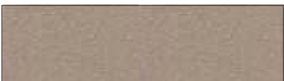
10 Colored Concrete, Light Broom Finish Denver Concrete - Sandstone (242) (Any exposed signage footers)
