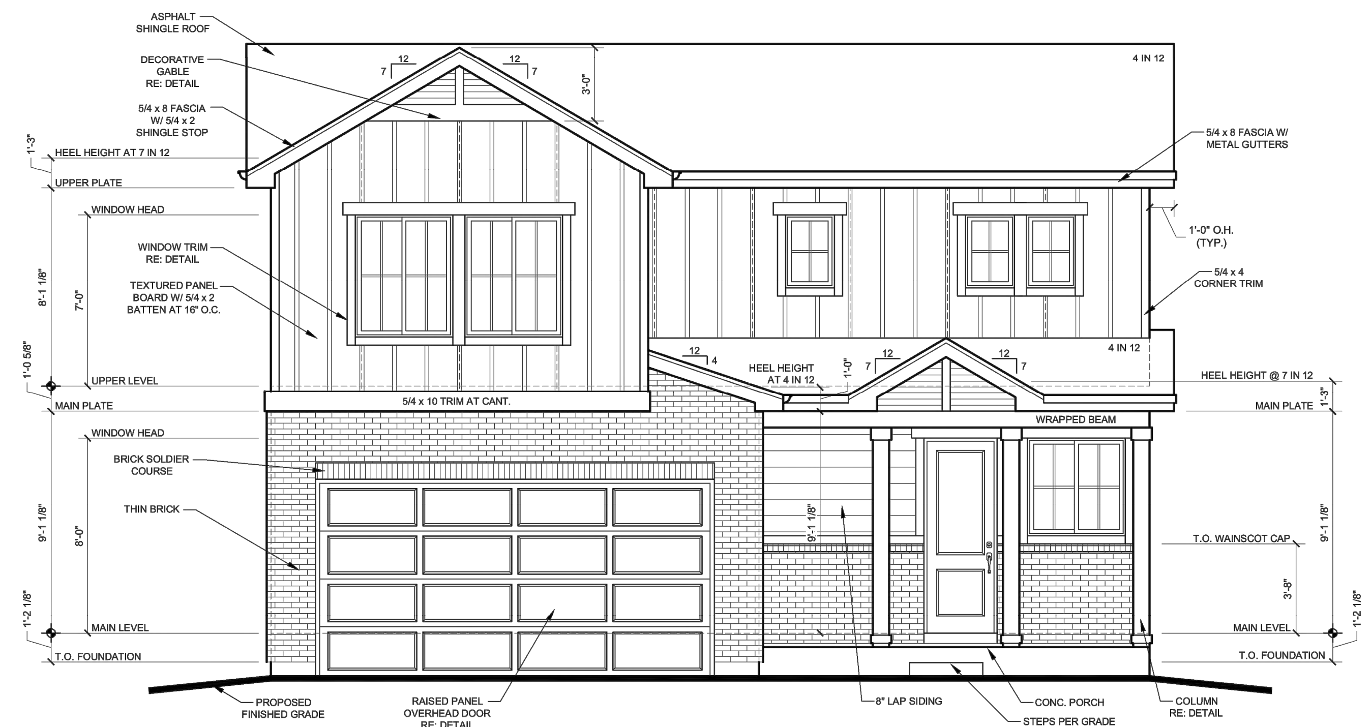
1 FRONT ELEVATION - 'A' FARMHOUSE 33% MASONRY 15% GLAZING SCALE: 1/4" = 1'-0"
