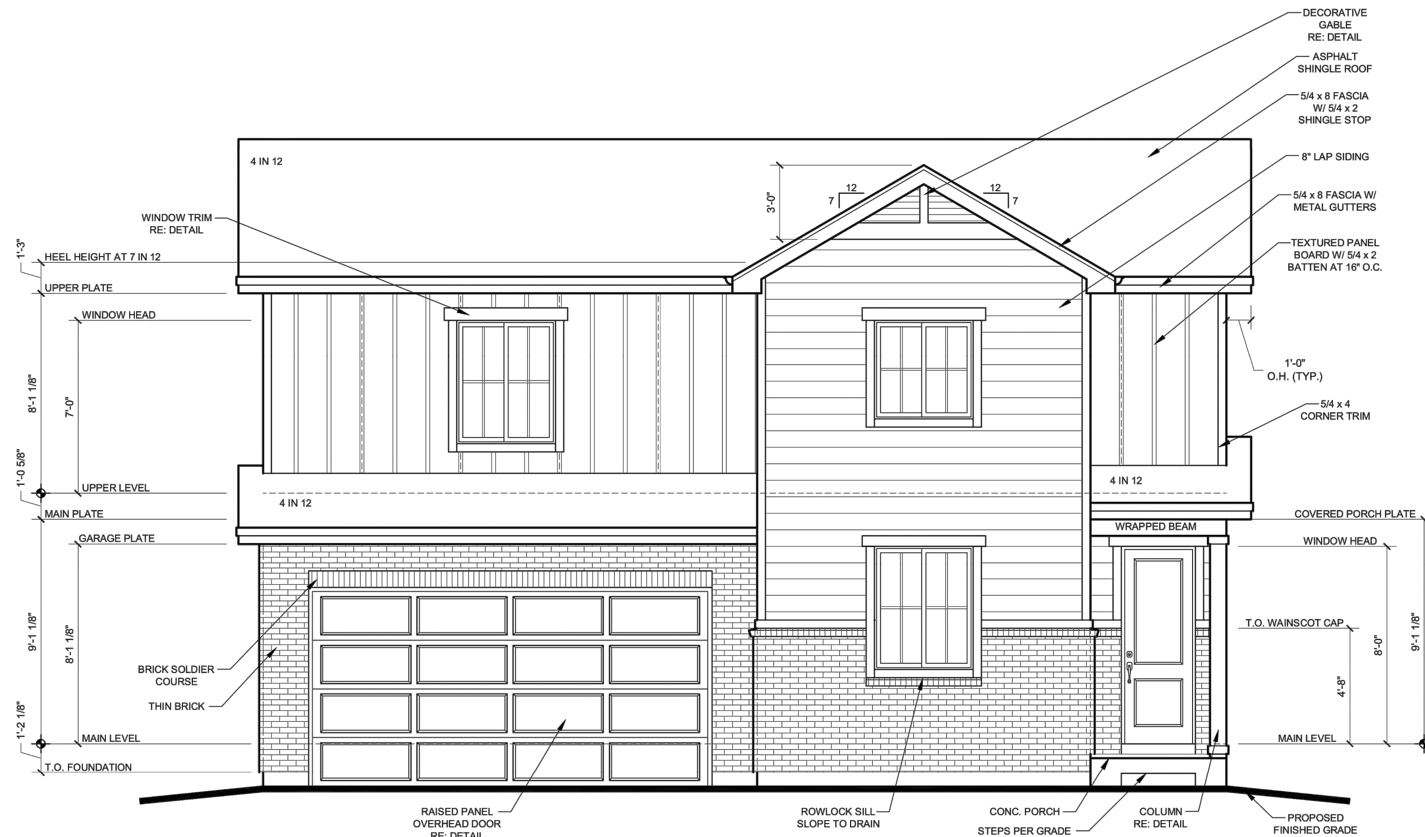
1 FRONT ELEVATION - 'A' FARMHOUSE 30% MASONRY 15% GLAZING SCALE: 1/4" = 1'-0"
