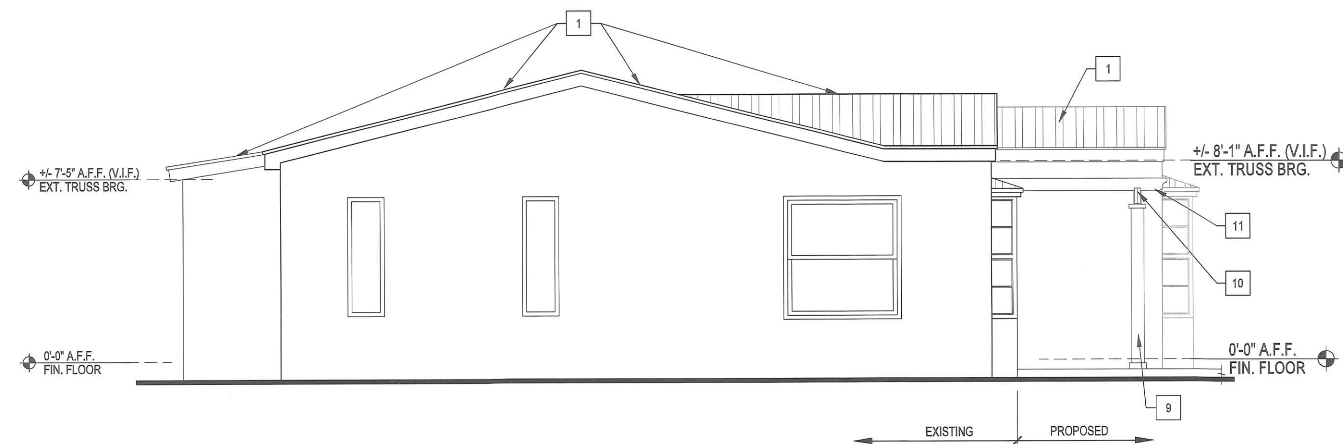
04 PROPOSED SOUTH ELEVATION SCALE: 1/4" = 1'-0"
