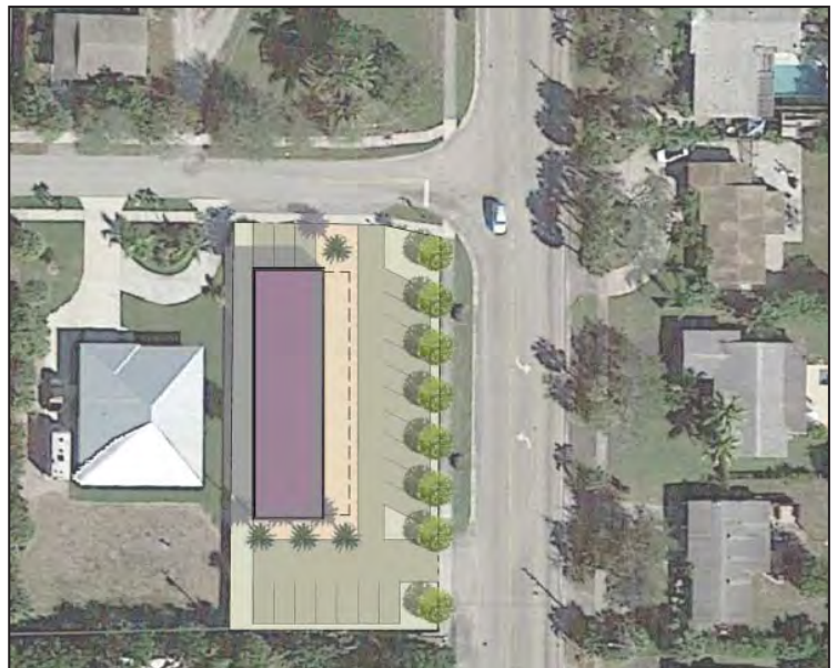
A revised site plan that creates a wide, shaded pedestrian area along the storefronts and adds a row of trees to shade the parking area and the sidewalk.
