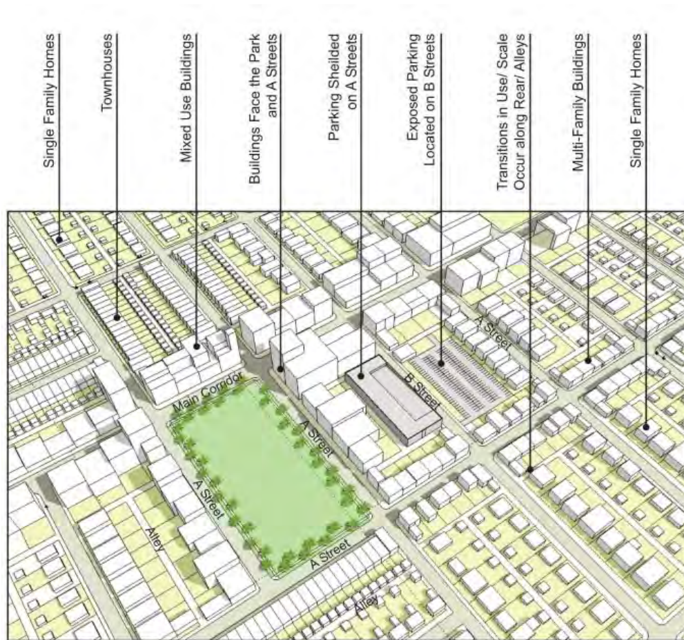
Illustration of transition of uses, scale, and massing. Note the use of roads and alleys in the transition between varying intensities.
