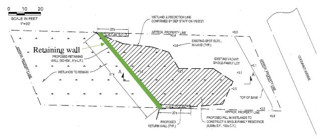
As you can see from the survey above, the area shaded in gray are jurisdictional wetlands that have been offset due to off-site mitigation. But the wetlands to remain are protected by a proposed retaining wall. Without this permit, the site would be practically unbuildable.
