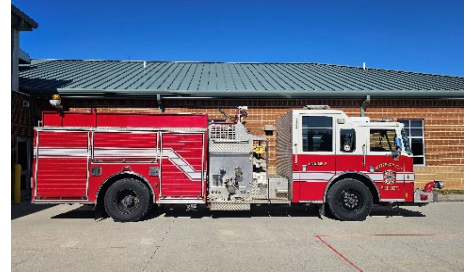
JCFD ENG 52 - Pumper (2003 Pierce Saber) 1500 PGM Pump, 1000 Gal Tank - In Service 28 Days
