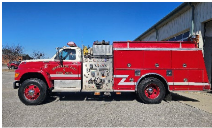
JCFD ENG 56 - Pumper (1997 KME Ford 700) 1250 GPM Pump, 1000 Gal Tank
