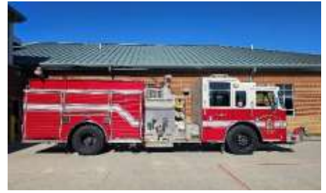
JCFD ENG 52 - Pumper (2003 Pierce Saber) 1500 PGM Pump, 1000 Gal Tank - In Service 31 Days
