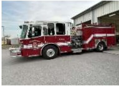
JCFD ENG 51 - Pumper (2013 Ferrara Ignitor) 1500 GPM Pump, 750 Gal Tank
