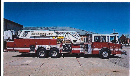
JCFD TRK 51- Aerial Ladder (2002 Ferrara Inferno) 2000 GPM Pump, 300 Gal Tank, 100' Aerial Platform -In Service 20 Days
