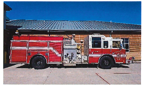
JCFD ENG 52 - Pumper (2003 Pierce Saber) 1500 PGM Pump, 1000 Gal Tank - In Service 31 Days
