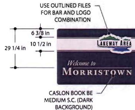
G3.1 TYPICAL SIGN FACE LAYOUT SCALE: 3/8" = 1'-0"
