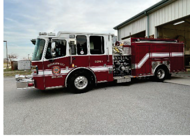
JCFD ENG 51 - Pumper (2013 Ferrara Ignitor) 1500 GPM Pump, 750 Gal Tank
