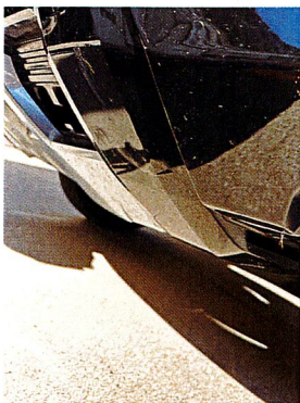
9/5/2025 Comments: REPLACE LOWER COVER LARGE CRACK
