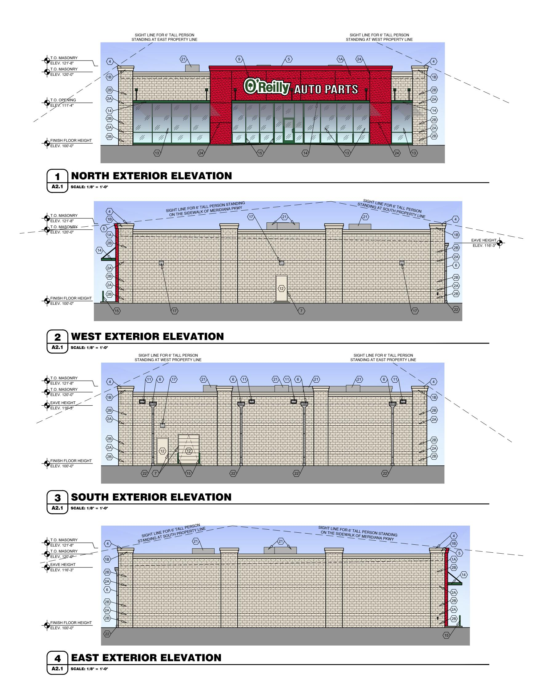
PORTLAND CEMENT STUCCO KEY NOTE NO. 1A: MFG: STO SPECIFIED. EQUAL BY DRYVIT OR MASTER BUILDERS (NO SUBSTITUTES) SERIES: STO POWERWALL TEXTURE: FINE COLOR: STUCCO TO HAVE INTEGRAL COLOR MATCHING SHERWIN WILLIAMS "POSITIVE RED" SW6871 (SHER-CRYL) GLOSS
