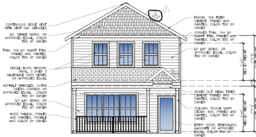
FRONT EXTERIOR 2A ELEVATION 1/4"=1'-0" 4' 6'
