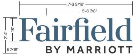
NON ILLUMINATED PIN-MOUNTED LETTERS SCALE: 1/2" = 1'-0"
