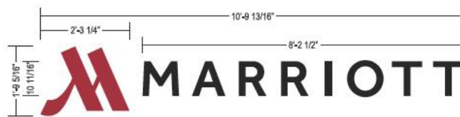
NON ILLUMINATED PIN MOUNT LETTERS DETAIL SCALE: 1/2" = 1'-0"
