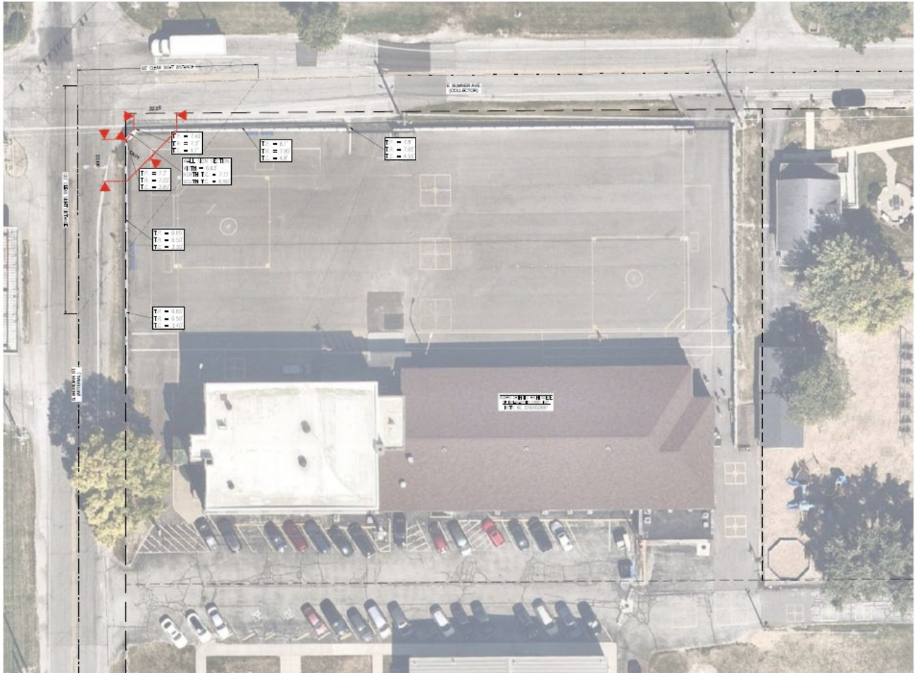
Site plan showing fence moved in roughly 16 feet from its current location
