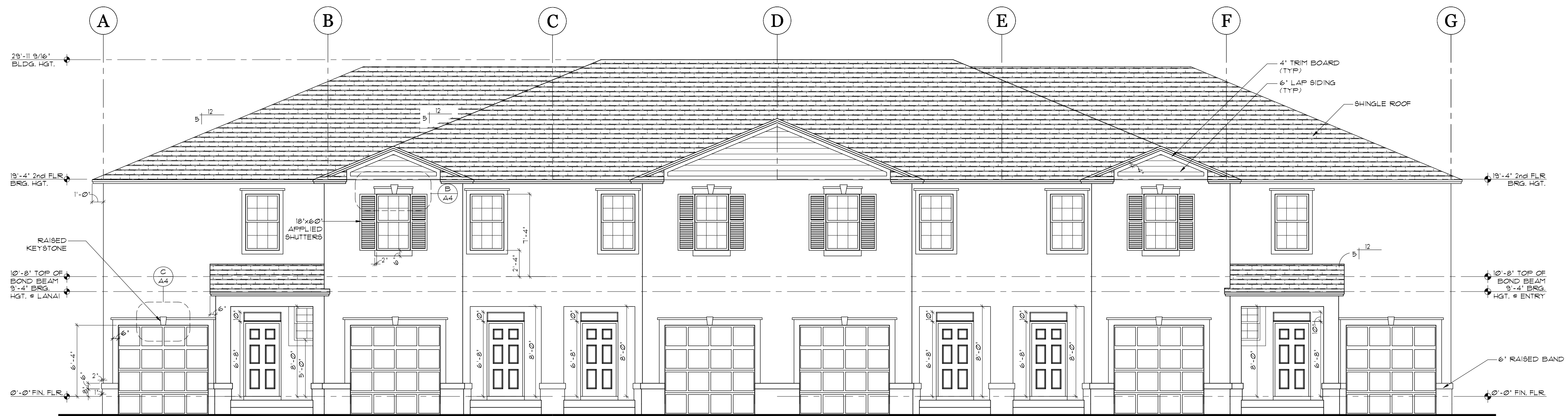
FRONT ELEVATION SCALE: 3/16" = 1'-0" TEXTURED FINISH NOTE: WALL PENETRATION FLASHING AS PER FBCR 103.4
