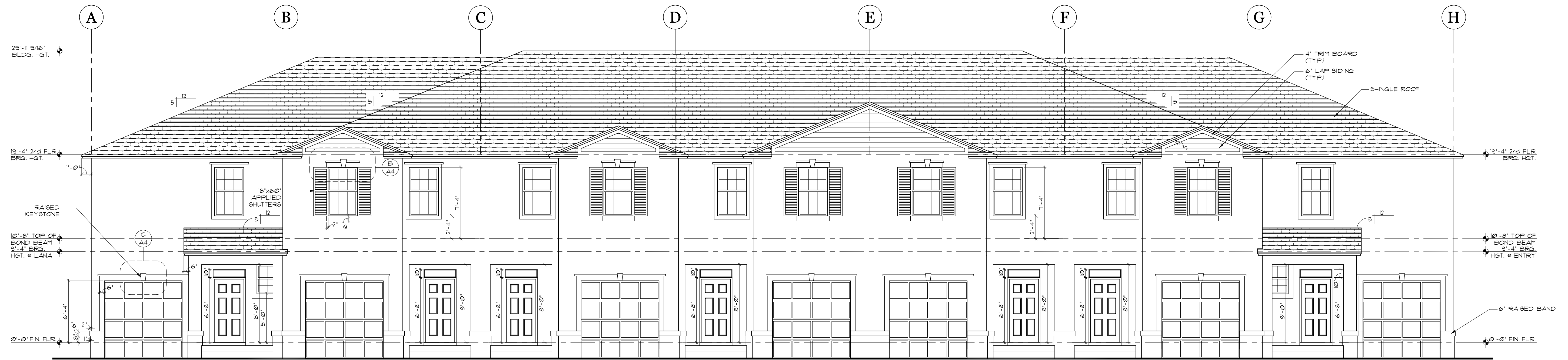
FRONT ELEVATION SCALE: 3/16" = 1'-0" TEXTURED FINISH NOTE: WALL PENETRATION FLASHING AS PER FBCR 103.4
