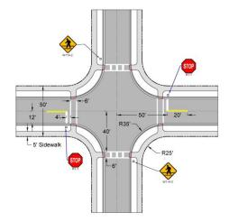
10. Identify on the plans the locations where sidewalks are to be constructed with the subdivision construction. Add a note that all curb ramps are to be constructed with the subdivision.
