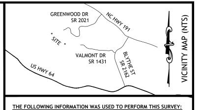
CLASS OF SURVEY: <u>CLASS A HORIZONTAL</u> POSITIONAL ACCURACY AT 95% CONFIDENCE: <u>0.02' (HORIZONTAL)</u> <u>0.03' (VERTICAL)</u> GPS/GNSS FIELD PROCEDURE: <u>STATIC (CARLSON SURVEY GNSS</u> DATE(S) OF SURVEY: 5/22/23 DATUM/EPOCH: NAD 83 (NSRS 2011) EPOCH 2010.00 (H) NAVD 88 (V) DATUM/EPOCH: <u>NAU 05 (11)</u> GEOID MODEL: <u>GEOID 18</u> FIXED CONTROL: <u>CORS (NCHE, NCSW, P779)</u> COMBINED GRID FACTOR(S): <u>0.99976754</u> (GNSS OBSERVED POINT) <u>0.99976051</u> (LOCALIZED POINT)
