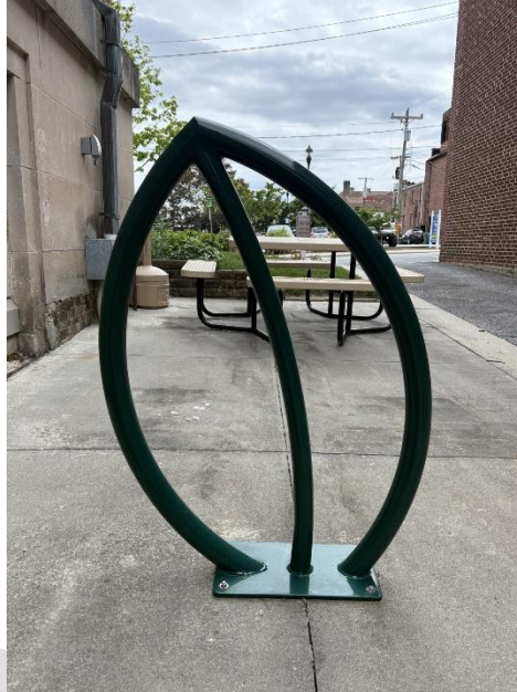
Figure 9: Example City of Hendersonville "leaf" bike rack. Bike racks of this nature provide two points of contact and accommodate two bicycle parking spaces each
