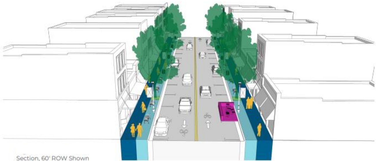
Figure 4: Example of Cross-Section from Downtown Master Plan for Streetscape Character Type "Downtown". Descriptions and cross-sections for each streetscape character type are found on pages 68-84 in the Downtown Master Plan.
