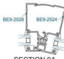
SECTION 9A 0°- 12.5° HINGED INSIDE CORNER
