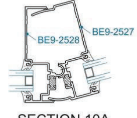
SECTION 10A 3°- 15° HINGED OUTSIDE CORNER
