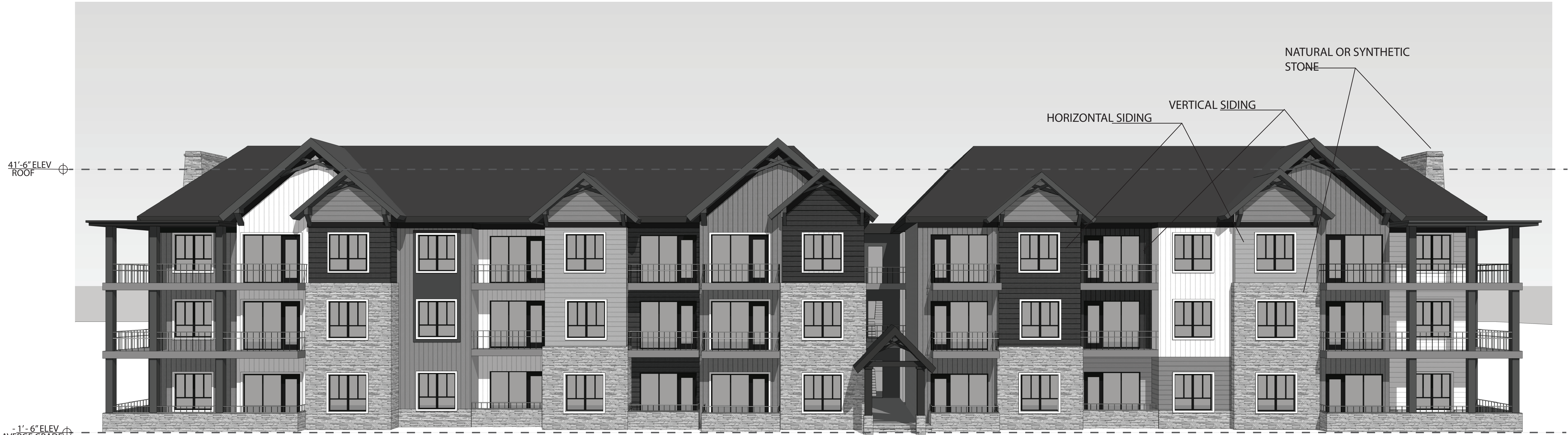
1 SOUTH ELEVATION | TYPICAL BUILDING SCALE : 1/8" = 1'-0"
