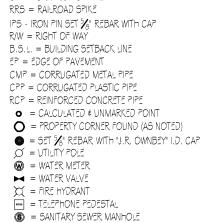
LEGEND: EIP = EXISTING IRON PIPE CTP = CRIMPED TOP PIPE
