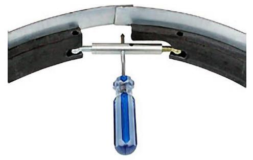
Our Manhole Adjusting Riser Rings feature a turnbuckle linkage pivoted at each end to provide the ultimate means to expand a manhole riser.
