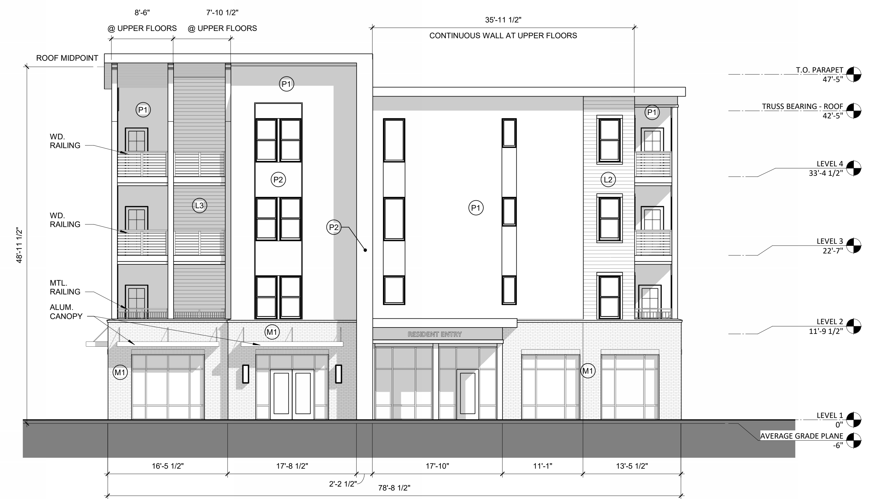
2 NORTH ELEVATION - LEASING ENTRY SCALE: 1/8" = 1'-0"
