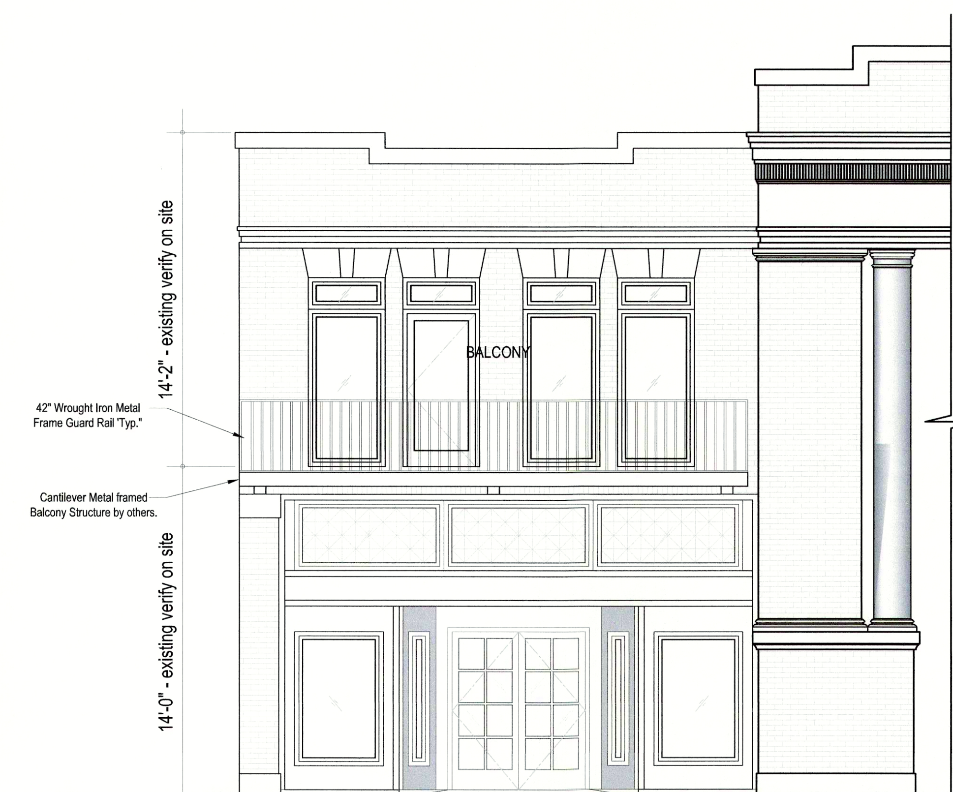
A RENOVATED FRONT ELEVATION Scale : 1/4" = 1'-0"
