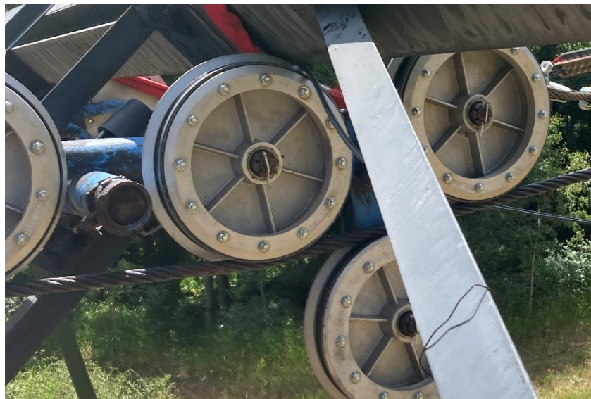
Figure 6 Sheave Assembly Against cross beam
