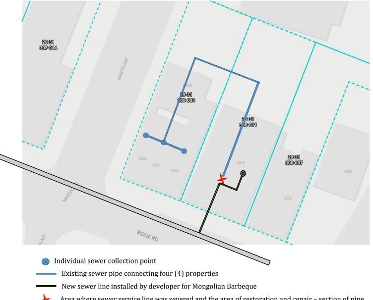
Area where sewer service line was severed and the area of restoration and repair – section of pipe was restored.
