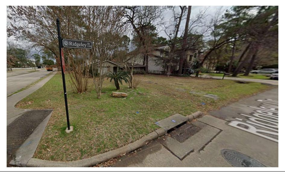
**Applicant Observation:** The stop sign, narrow lot, and transition from curb and gutter drainage system to open ditch drainage system present many design issues.
