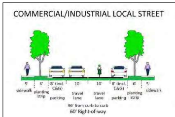
TYPICAL PUBLIC STREET SECTIONS TO BE USED IN PROJECT SCALE: NTS
