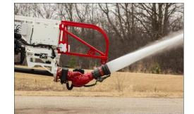
When the aerial device is positioned at -10 to 0 degrees of elevation, the master stream will be capable of flow up to 30 degrees above horizontal.
