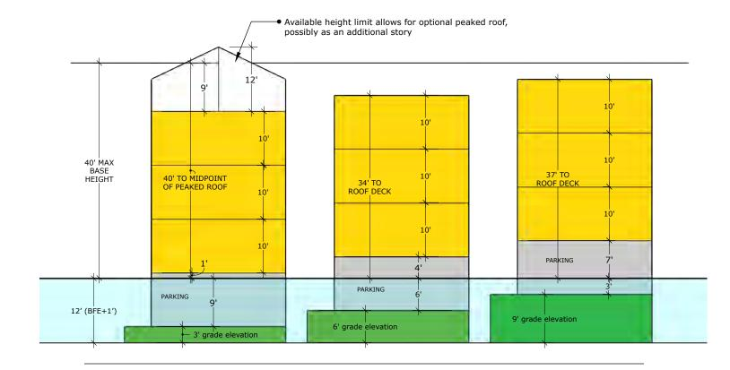
Illustration of Building Heights at three different grade elevations. Height is measured from BFE+1 = 12 feet.
