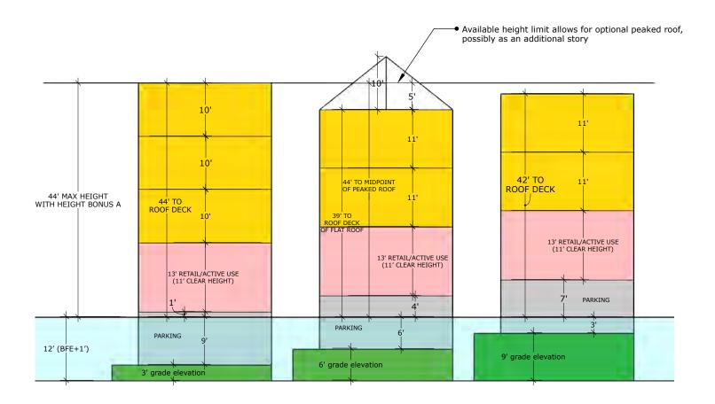
Illustration of Building Heights at three different grade elevations. Height is measured from BFE+1 = 12 feet.
