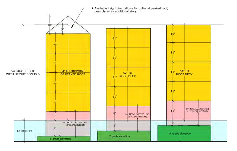
Illustration of Building Heights At three different grade elevations. Height is measured from BFE+1 = 12 feet.
