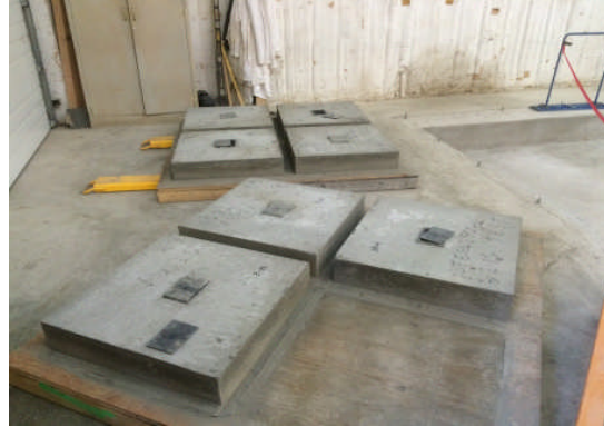
Concrete Blocks with Forms Removed
