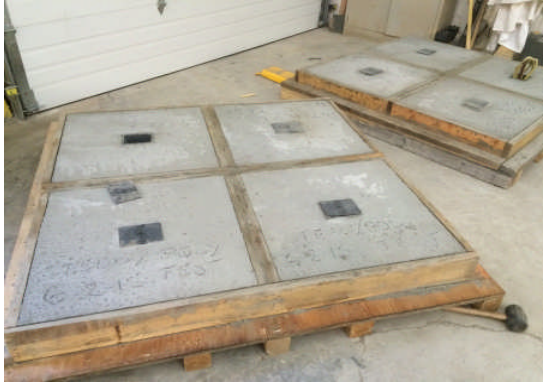
Concrete Blocks as Received (Plywood Lid Removed)
