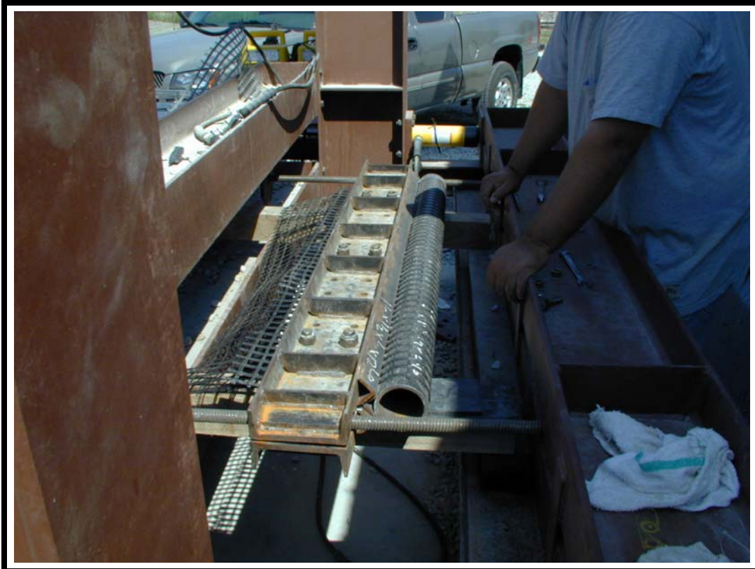
PHOTO NUMBER 2 Geogrid Pullout System
