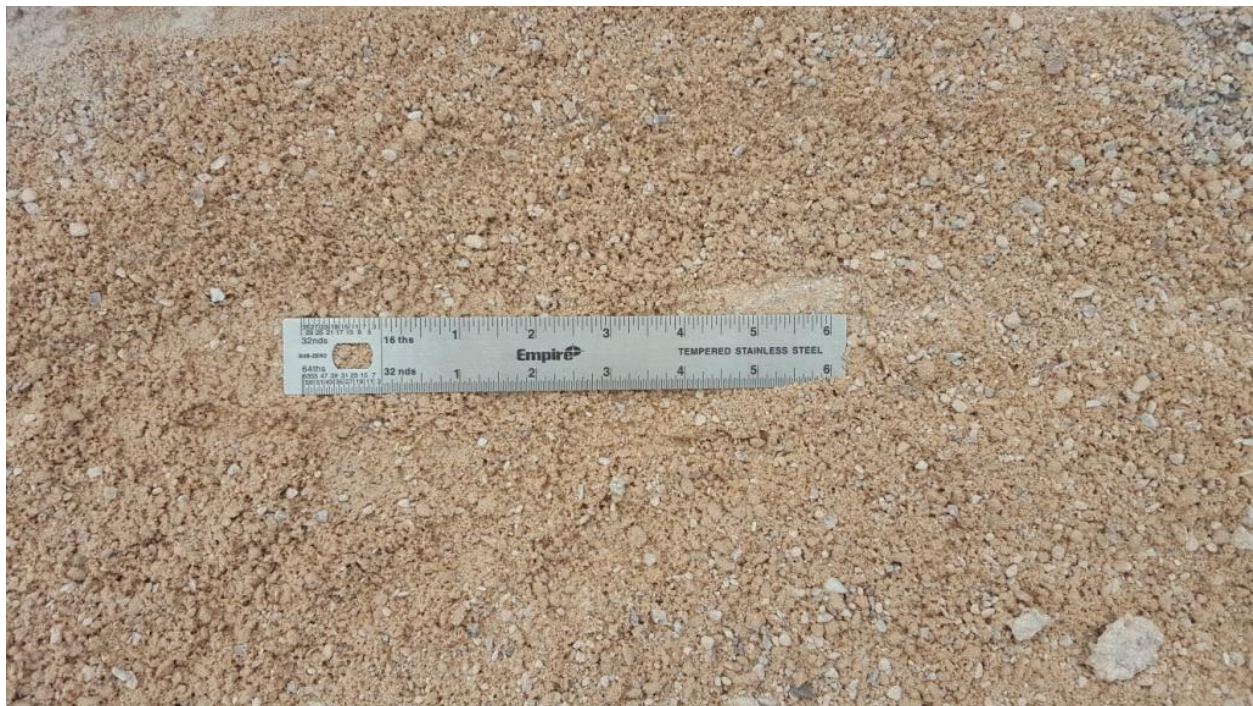
Figure 4-4. Installation damage Type 3 test aggregate.
