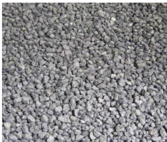
Figure E-2. ISO/EN 10722, laboratory installation damage aggregate.
