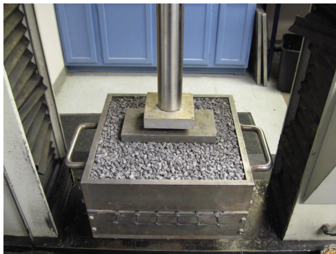
Figure E-1. ISO/EN 10722, laboratory installation damage test apparatus.
