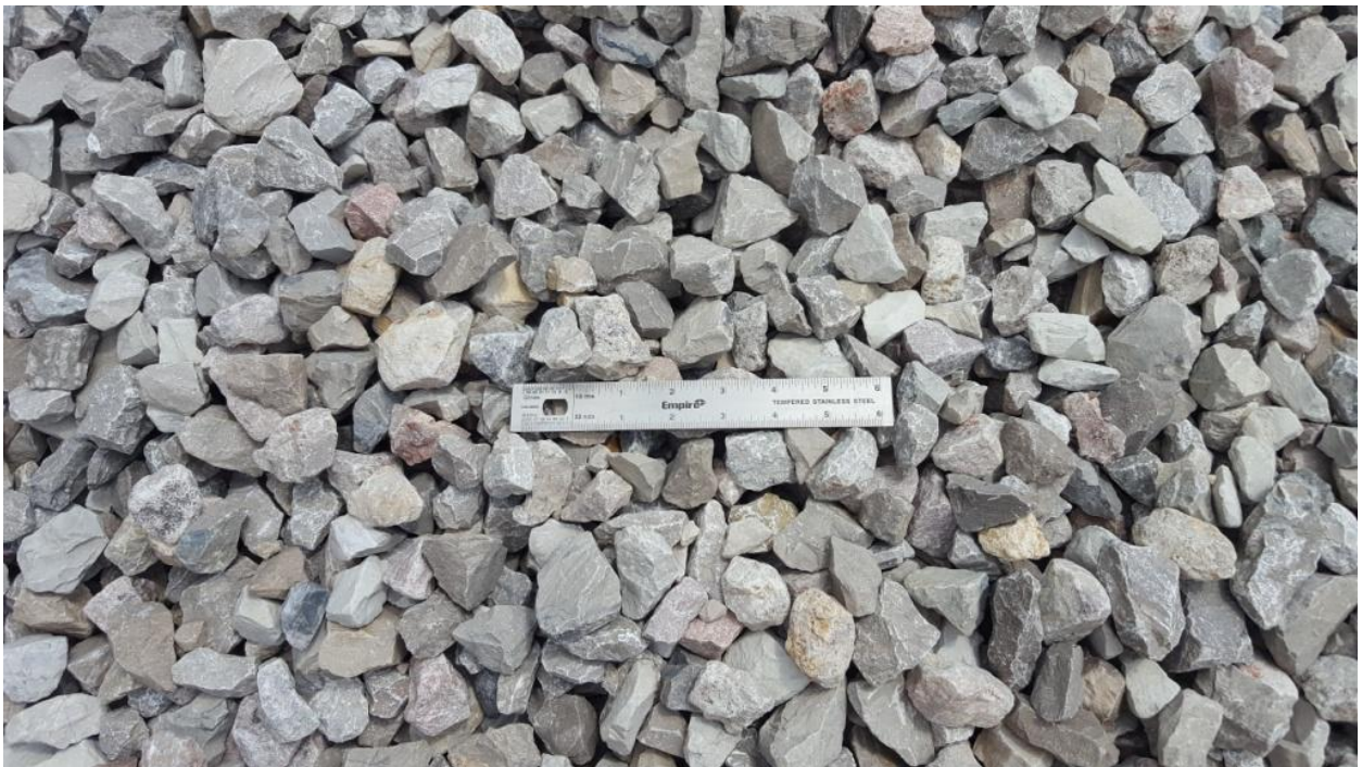
Figure 4-2. Installation damage Type 1 test aggregate.
