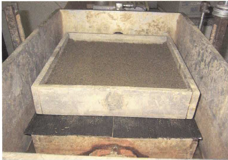
Figure 2. Soil placed in the upper shear box and compacted on top of Parawebs to a specified unit weight
