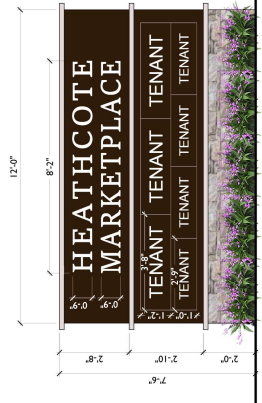
2 SECONDARY SIGNAGE = 36 SF PER SIDE / 72 BOTH SIDES (100 SF MAX) NOTES: THIS DRAWING HAS NOT BEEN REVIEWED BY A STRUCTURAL ENGINEER. REFER TO STRUCTURAL SIGNAGE MATERIALS AND ILLUMINATION MAY VARY BUT WILL BE IN GENERAL CONFORMANCE TO WHAT IS SHOWN HERE.
