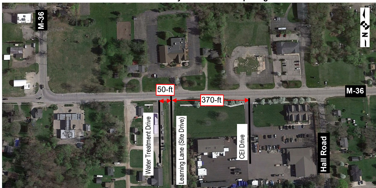
Exhibit 1: Driveway & Intersection Spacing
