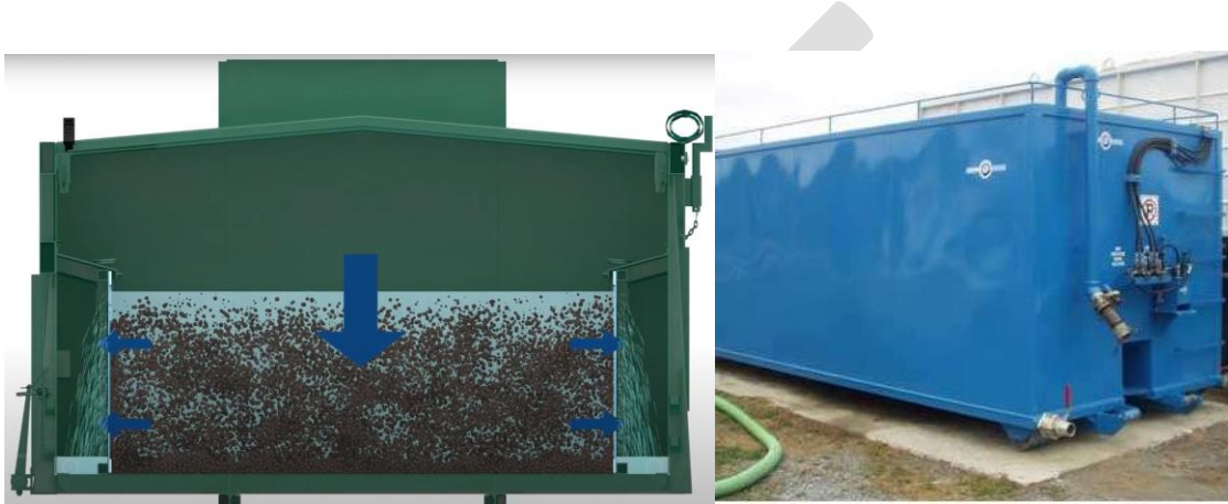
Figure 11. Dewatering Container Schematic and Exterior
