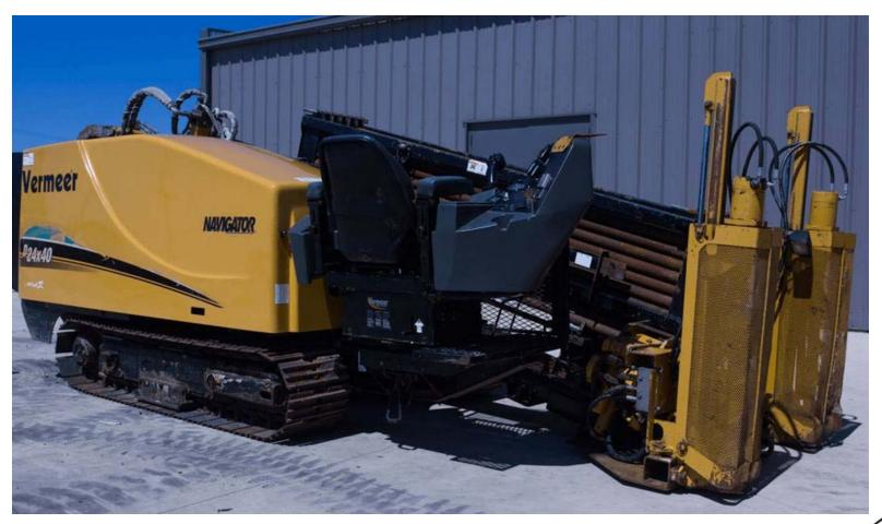
Directional boring machine. Crossings below the road ROW would also be accomplished by boring.
